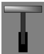
**T-Bar** — enables you to perform smooth, manual transitions. Each time the **T-Bar** is moved from limit to limit, the “look” on Preview transitions to Program using the selected transition type (as chosen on the **Effects Menu**).
